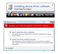
**NOTE**: The Ambulo 2400 USB driver is unsigned. To successfully install the Ambulo 2400 USB driver on certain Windows operating systems such as Windows 8.1, it is necessary to temporarily disable the driver signature enforcement of Windows prior to successful installation. Please refer to the Microsoft Windows technical documentation and instructions or relevant articles available on the Internet as to how to perform this task.
